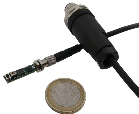
Fig. 2: Variant A demonstrator and EMC test board
