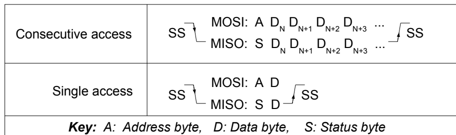
Fig. 7: Single byte and sequential byte accesses
